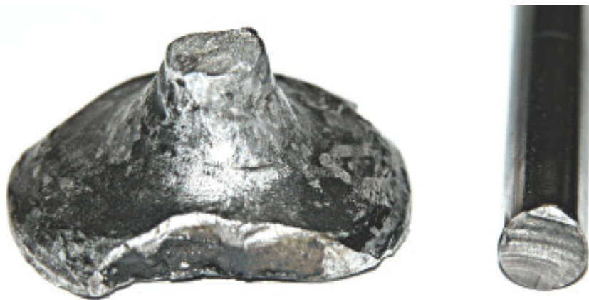
Photo 1. Typical valve stem fracture at the underhead radius and stem junction. The stem fracture face is usually in good condition, while the valve head fracture face is typically too damaged to be of use.
