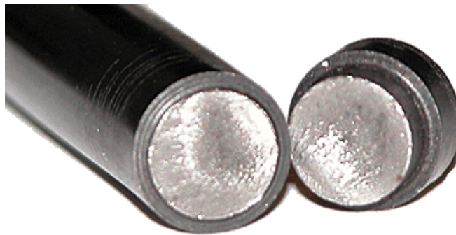
Photo 2. Valve stem fracture at the collet groove. The fracture shows no sign of cyclic fatigue, but the stem end is bent and the fracture face is typical of high overstress.
