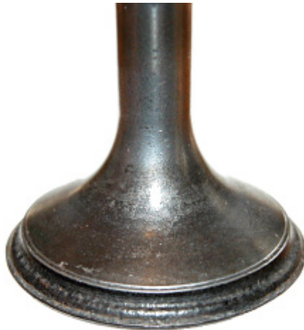
Photo 1. Valve face wear or guttering.
