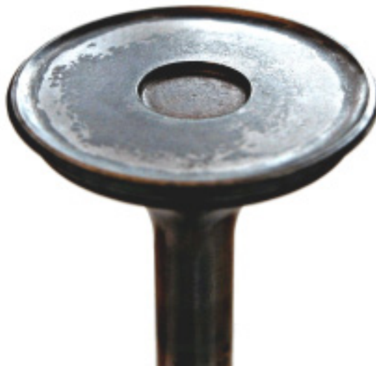
Photo 2. Valve head cupping or tuliping.
