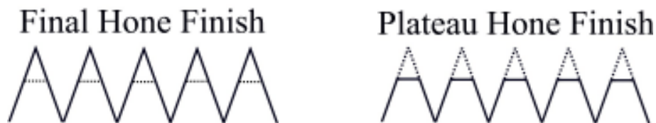
Figure 1. Final hone and plateau hone profile.
