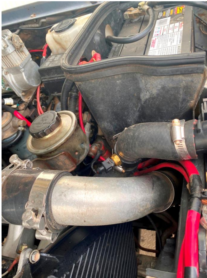
Radiator inlet and outlet temperature sensors for measuring temperature drop across the radiator in real time.
